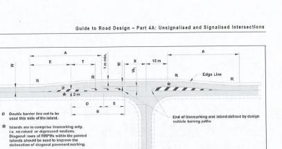
Note: The dimensions of the treatment are defined below and values of A, D, R and T are shown in Table 7.1:
